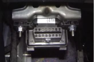
On the back of the DLC module there is a wiring connector that contains the required CAN signals for the CB-2 CAN Interface. The CB-2 should be connected to the DLC module as outlined in the following table.
