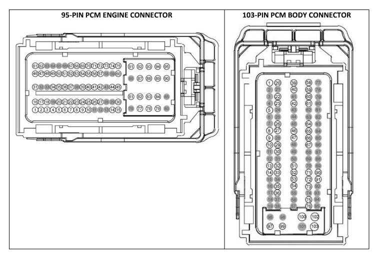
The Cortex EBC wiring harness can be connected to the PCM connectors as outlined in the following table (B = Body Connector, E = Engine Connector). RPM and vehicle speed signals are required for boost by gear applications.
