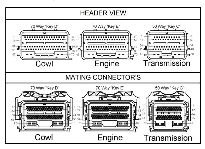
The Cortex EBC wiring harness can be connected to the PCM connectors as outlined in the following table (C = Cowl Connector, E= Engine Connector, T = Transmission Connector). RPM and vehicle speed signals are required for boost by gear applications.
