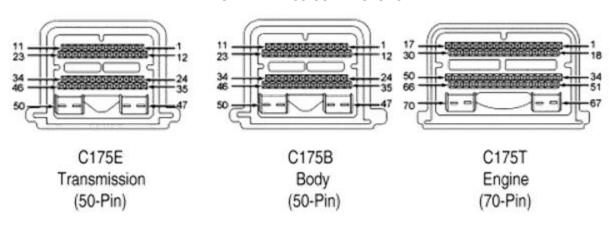
The Cortex EBC wiring harness and Speed Sensor Adapter V2 can be connected to the PCM connectors as outlined in the following tables (B = Body Connector, E= Engine Connector, T = Transmission Connector). RPM and vehicle speed signals are required for boost by gear applications. The Speed Sensor Adapter V2 can be connected to the same power and ground source as the Cortex EBC if desired.
