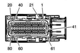
The Cortex EBC wiring harness should be connected to the 80-pin X2 ECM connector as outlined in the following table.
