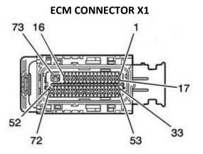
The Cortex EBC wiring harness should be connected to the 73-pin X1 ECM connector as outlined in the following table.
