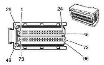
The Cortex EBC wiring harness should be connected to the 96-pin X1 PCM connector as outlined in the following table.
