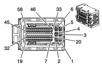
The Cortex EBC wiring harness should be connected to the 58-pin X2 PCM connector as outlined in the following table.
