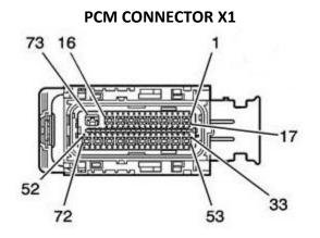
The Cortex EBC wiring harness should be connected to the 73-pin X1 PCM connector as outlined in the following table.
