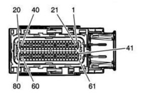
The Cortex EBC wiring harness should be connected to the 80-pin X2 PCM connector as outlined in the following table.
