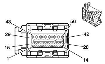
The Speed Sensor Adapter should be connected to the 56-pin C3 PCM connector as outlined in the following table. The adapter can be connected to the same power and ground as the Cortex EBC.
