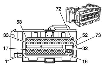
The Cortex EBC wiring harness should be connected to the 73-pin C2 PCM connector as outlined in the following table.
